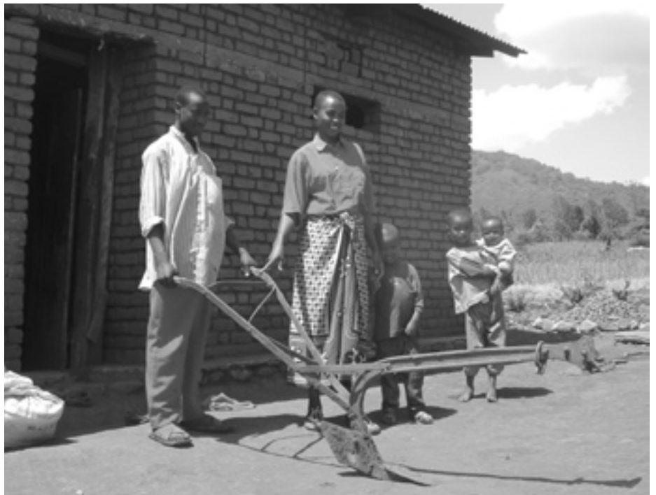
A family outside their house with a Magoye Ripper, an effective and low cost implement introduced by the LAMP project to rip through the soil hardpan.
